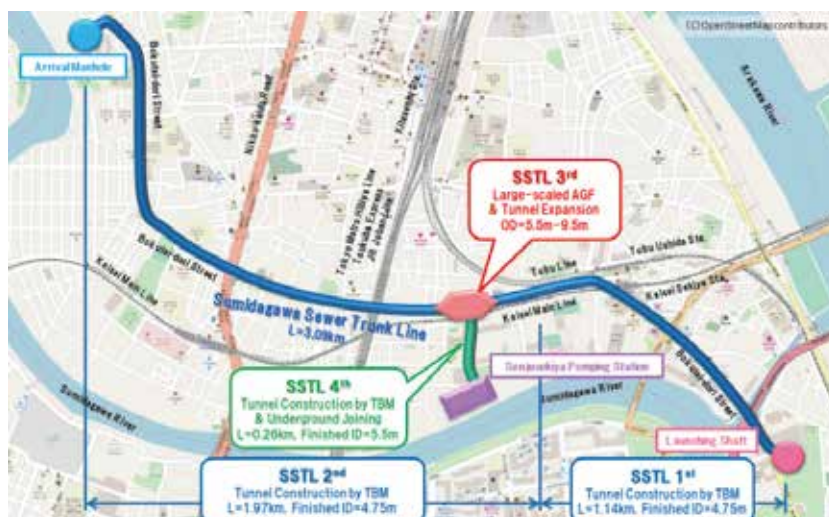
Fig.4 The Sumidagawa Sewer Trunk Line
